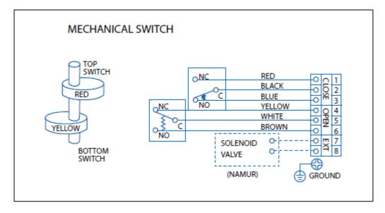
Wiring scheme for mechanical switches
