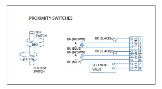
Wiring scheme for proximity switches
