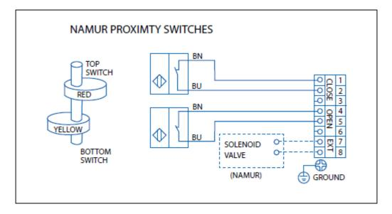
Wiring scheme for NAMUR proximity switches
